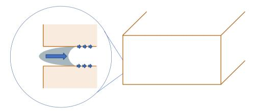
The large pore structure of these bricks ensures that they can never freeze and break into pieces, even when they are saturated with water, as there is always sufficient space for the water to expand when it turns into ice.
